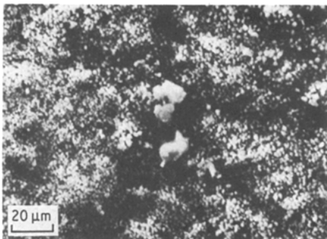
Figure 6 SEM view of a corroded zinc surface in pH 11 and NaClO 2 (10 g litre -1 ) solution for 16 h.
